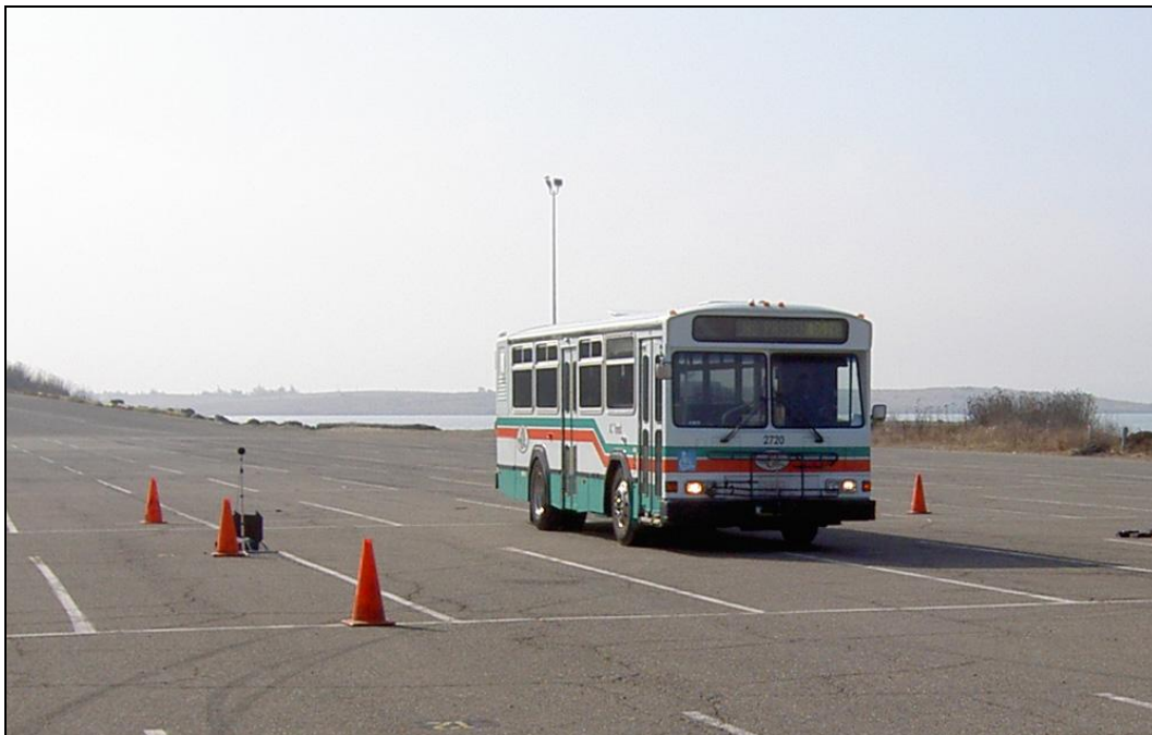
Figure 21: Photograph of Gillig Bus During Controlled Noise Measurements
