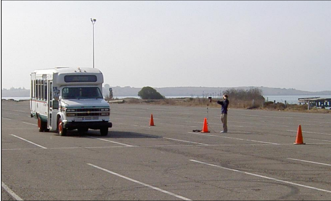
Figure 22: Photograph of Gas Van During Controlled Noise Measurements
