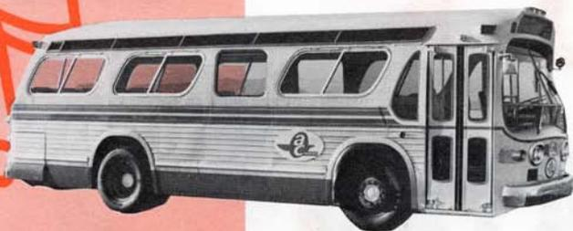
To obtain a reliable small bus, suitable for efficient operation of a Dial-A-Ride system, AC Transit cut down a regular 35-foot coach seating 45 passengers.
